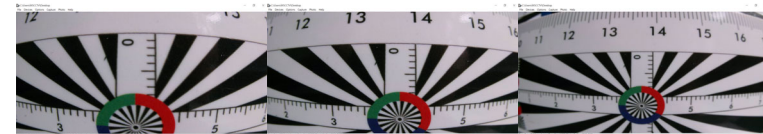
▲ High DOF (using 36060 lens, FID 20–15–30)
